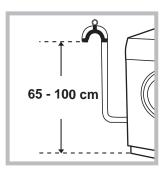
Connect the drain hose, without bending it, to a draining duct or a wall drain situated between 65 and 100 cm from the floor;
